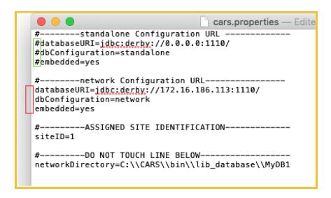
10. Still in the **cars.properties** file, replace the IP address highlighted in the image below with the IP address that is linked to the main networked computer. Replace only the numbers that are highlighted.
